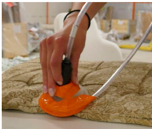
Figure 2. Push-pull method, used for difficult to clean, porous surfaces. Air is blown into the dome-shaped handpiece (right tube) and pulled out vertically through the black testing tube
