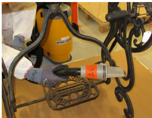
Figure 1. Clearance testing, vacuum-cleaner method: 2 m 2 of surface was sucked onto a glass-fiber filter. The filter number was written on the nozzle
