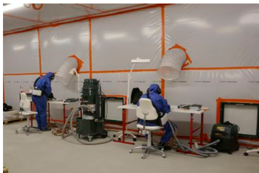
Figure 6. Cleaning zone with the extraction hose above and at floor level next to the worktables
